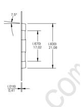
1. ALL TAPE & SPROCKET HOLE DIMENSIONS ARE PER EIA-481 UNLESS NOTED 2. ALL POCKET DIMENSIONS ARE ±(.004') 0,10mm 3. ALL DIMENSIONS ARE TO INSIDE OF POCKET
